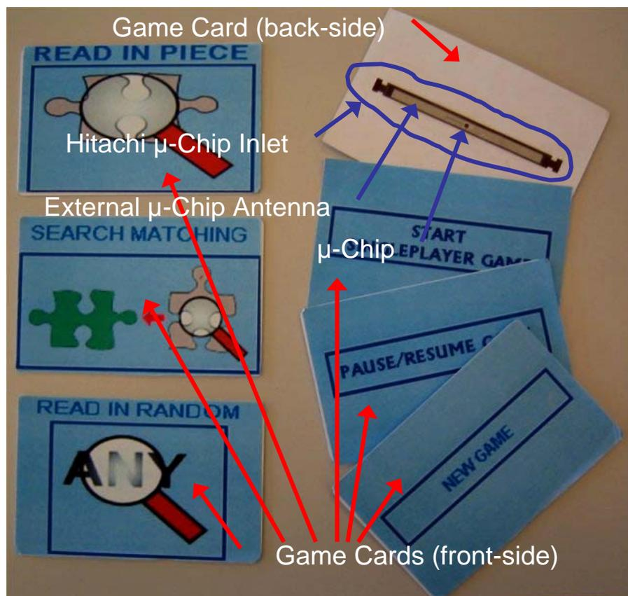
**Figure 2:** Game cards of the Smart Jigsaw Puzzle Assistant, tagged with RFID tags (Hitachi  $\mu$ -chip inlets) on the back-sides. In the top right of the photo, one can discern the external antenna and the tiny  $\mu$ -chip of a  $\mu$ -chip inlet
