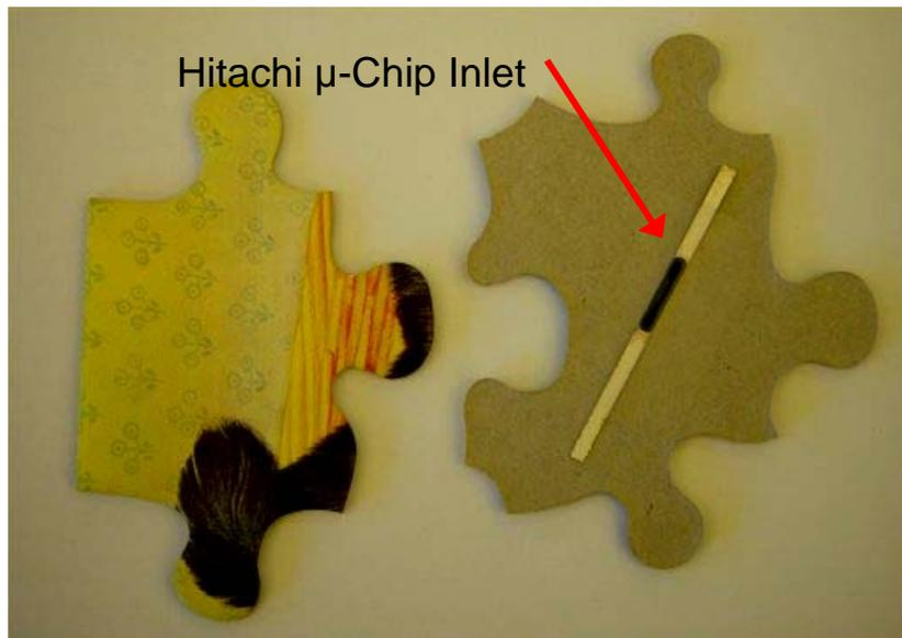
**Figure 3:** Two pieces of the tagged puzzle game. On the left the front-side view of a tagged piece is shown. On the right, one can see the back-side of a matching piece with an attached miniature RFID tag (Hitachi  $\mu$ -chip inlet). The Hitachi  $\mu$ -chip inlets we used for our SJPA prototype consist of a  $\mu$ -chip with a size of 0.4 mm square and an external antenna
